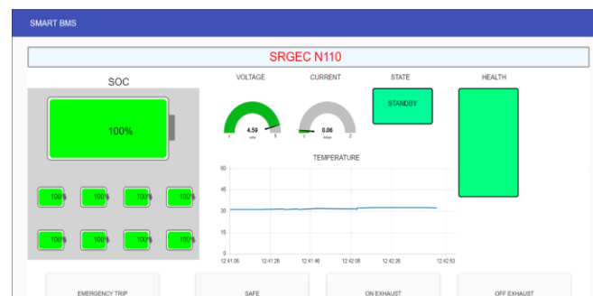
Fig. 11. Local BMU (Battery Monitoring Unit)
